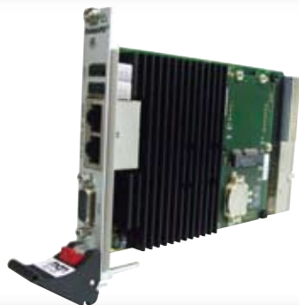
Intel Model: F21P ◇Intel ◇2.0~3.0GHz ◇Core i7 2nd gen ◇~16 GB DDR3 Core i7搭載CompactPCI PlusIOボード
