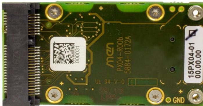
The PX4 is a PCI Express® Mini Card providing an audio and sound interface for mobile wireless functions. It can be equipped with an additional PCI Express® Mini Card with UMTS, LTE, GPRS and Edge for mobile phone functionality.
