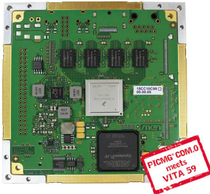
The CC10C is a Rugged COM Express® module (RCE) built around the Freescale™ ARM® i.MX 6 series of processors with a Cortex®-A9 architecture. Supporting different types of the i.MX 6Solo, 6DualLite, 6Dual and 6Quad families, the computer-on-module is widely scalable, e.g., to processing or graphics requirements. Where less performance is needed, you can optimize costs by choosing a single- or dual-core processor instead of a quad core.
