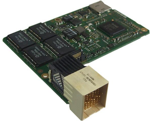
The GM1 is a mezzanine card which is plugged onto CompactPCI® Serial CPU boards to implement four Ethernet interfaces on the backplane. The CompactPCI® Serial standard defines up to eight Ethernet interfaces which can be connected in a star or
