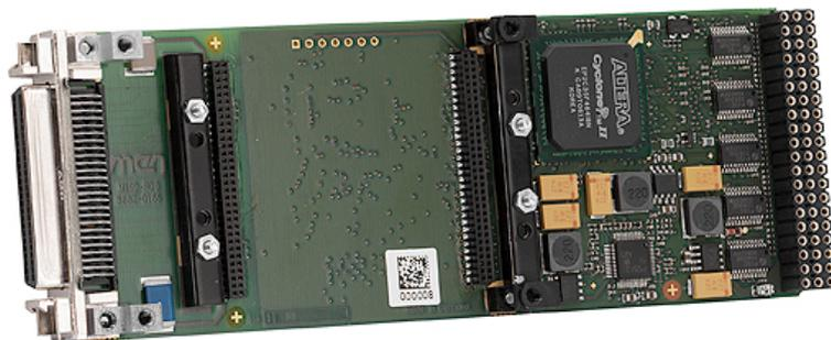
USM Universal Submodules make M-Modules more flexible than ever. The main M-Module M199 mezzanine card gets its specific function through the IP cores implemented inside its onboard FPGA. This function can be changed at any time through implementation of different IP cores. The corresponding line drivers are realized on the USM which is simply plugged on the M199.
