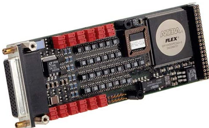
The M72 M-Module is a timer, counter and comparator with four 32-bit counter units. The four counters work independently in several modes, e.g. counting decoder signals or measuring frequencies. Each counter can be loaded with a preset value and can generate several events. Events can set or reset output signals, which are optically isolated.
