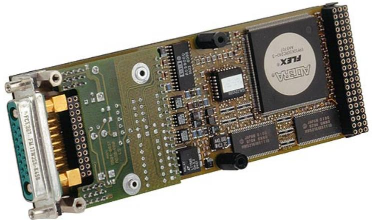
The mezzanine card M67 is a board for acquisition of analog signals with a bandwidth of up to 10 MHz at a maximum resolution of 12 bits and a sampling frequency of up to 40 MHz. Variable trigger functions allow application of the M67 as a "digital storage oscilloscope" for measurement and analysis applications.
