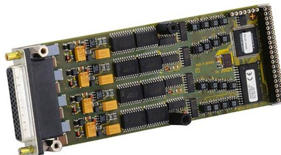
The mezzanine card M66 provides 32 binary process signals on one single M-Module, which is the largest number of binary channels ever seen on a mezzanine board. This allows a total of 128 signals with four M-Modules on a double Eurocard (i.e. in one slot of a VME or CPCI system). With its extremely high output
