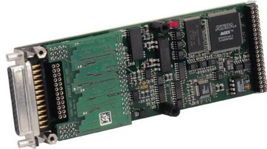
The mezzanine card M35N is a 14-bit analog M-Module for a wide range of standard input requirements such as 16 channels single-ended voltage or current and 8 channels differential voltage or current. The isolated supply voltages are generated by an onboard DC/DC converter, which is also usable in the extended temperature range of -40 to +85°C. A fast A/D converter and auto-incrementation of the
