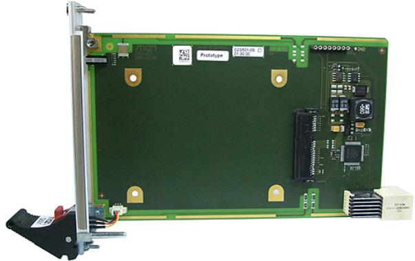
The G501 is a CompactPCI® Serial hard disk drive carrier board. It is designed to carry a 2.5" SATA hard
