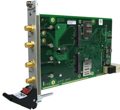
The G212 is a rugged single Eurocard CompactPCI® Serial carrier board supporting the PCI Express® Mini Card standard or, as an option, the ExpressCard® standard. ExpressCard® is the successor of the CardBus standard and offers different construction sizes as well as connection via PCI Express® or USB 2.0. The standard version of the G212 offers two PCI Express® Mini Card slots. It allows to use all types of cards for HF applications, for example GPS, WLAN,
