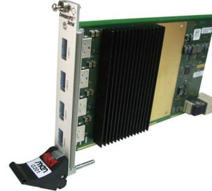
The G201 is a CompactPCI® Serial peripheral board offering four USB 3.0 host interfaces with a data rate of up to 5 Gbit/s per direction per port (2.28 Gbit/s measured). It can be used in combination with a CompactPCI® Serial or CompactPCI® PlusIO CPU board in a CompactPCI® Serial or hybrid system. It is
