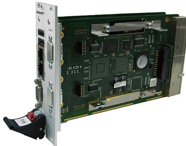
The F608 is a 4HP SATA extension card for 3U Intel® based CompactPCI® single-board computers. It can be used in combination with the F14 and [compatible CPU boards](#).
