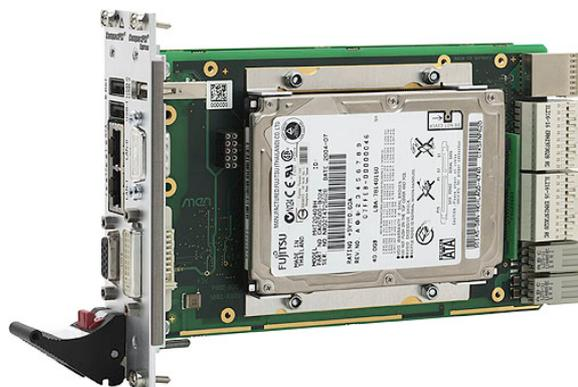
The F602 is a 4HP CompactPCI® Express extension card for 3U Intel®-based CompactPCI® single-board computers. It can be used in combination with the F14, F15, F17 and F18 CPU boards. That way, these CPU boards can be used both as system-slot cards in a CompactPCI® environment and as system-slot cards on a CompactPCI® Express backplane.
