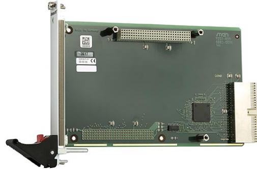
The F207 is a 3U CompactPCI® bus card which provides a PCI-104 interface supporting up to four PCI-104 extension boards. An on-board PCI-to-PCI bridge provides a 32-bit PCI interface at the PCI-104 connector and a 32-bit/33-MHz interface to the CompactPCI® bus. V(I/O) voltage is 3.3V on the local bus (5V on request) and 3.3V or 5V on CompactPCI®.
