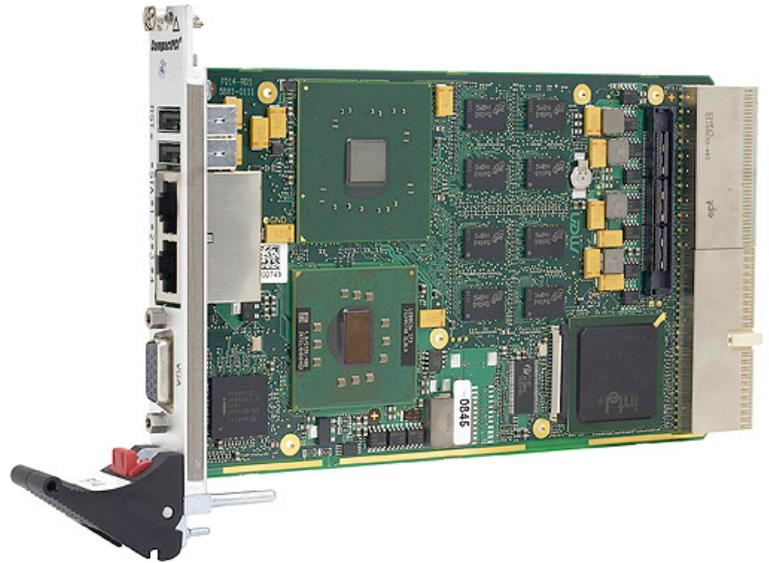
Equipped with the Intel® high-performance Core 2 Duo processor T7500 running at 2.2 GHz, the F18 is a versatile 4HP/3U (single-slot, single-size Eurocard) single-board computer based on the latest multi-core processor architecture from Intel® with full 64-bit support. The CPU card delivers an excellent graphics performance and is designed especially for embedded systems which require high computing performance with low power consumption.
