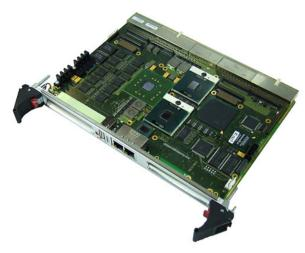
The D7 is equipped with two high-performance Intel® multi-core Xeon® processors, which consist of four CPU cores running at 1.66 GHz. The versatile 4 or 8HP/6U (single or double-slot, double-size Eurocard) CompactPCI® single-board computer is designed especially for embedded systems which require high computing performance. It comes with a tailored passive heat sink - forced air cooling is required inside the CompactPCI® system.
