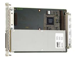
The B202S is an M-Module™ carrier board for universal peripheral input/output applications on the VMEbus. M-Modules™ are screwed tightly on the carrier board,
