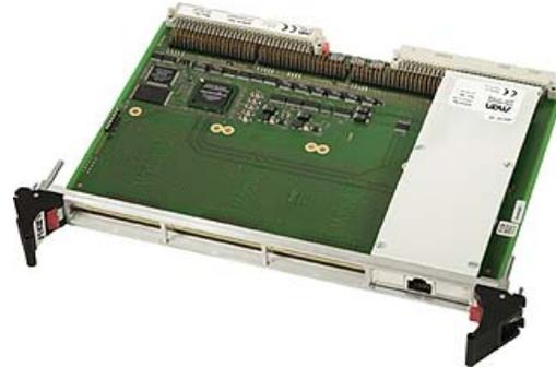
The A203N is an M-Module™ carrier board for universal I/O on the VMEbus, allowing high flexibility in applications such as process and motion control, measurement and instrumentation, communication or special-purpose tasks. The M-Modules™ are screwed tightly on the carrier board, and the board needs only one slot on the VMEbus.
