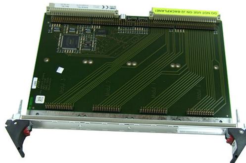
The M-Modules™ are screwed tightly on the carrier board, but the board needs only one slot on the VMEbus. Please note that since all three rows of the P2 connector are used for user I/O, board models with this connector are not compatible with VME64 backplanes.
