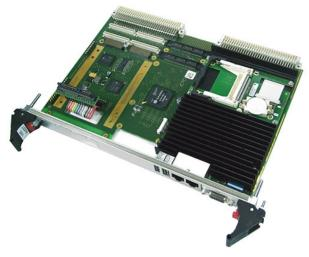
The A19 6U single-slot VMEbus SBC supports a variety of Intel® Core™ Duo and Core 2 Duo processors from the high-end 2.16 GHz T7400 to the low-voltage dual-core versions down to a selection of single-core Celeron® M types. It is designed especially for systems which require high computing and graphics performance and low power consumption in a typical Windows® environment or under VxWorks®.
