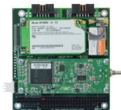
Janus-MM with GPS and Wireless modem Modules Installed
